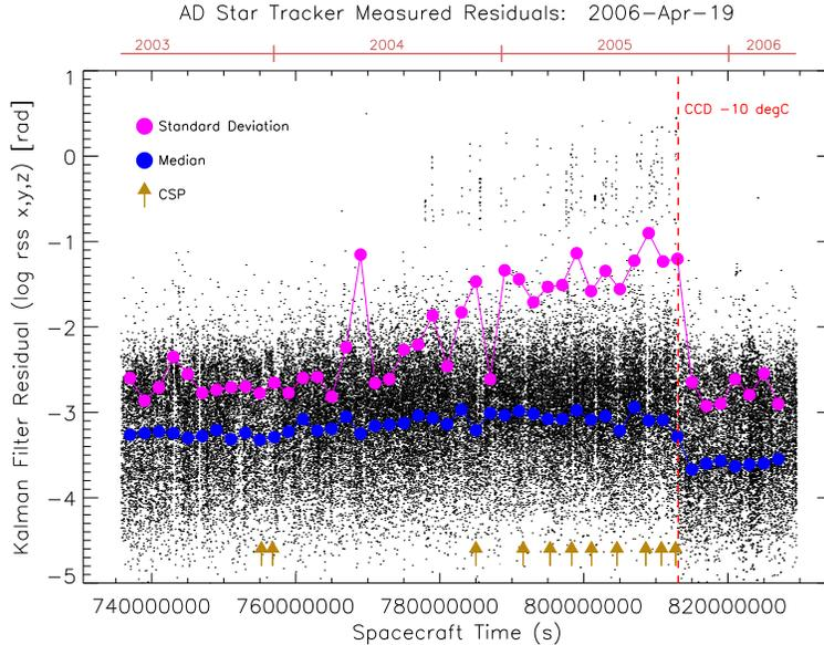
**Figure 7.** Tracker residuals for the GALEX mission showing the CSP events (arrows) and the improvement in noise performance after cooling the tracker CCD from 0 to  $-10^{\circ}\text{C}$ . The onset of high-residual events occurred quite rapidly about midway through 2004.
