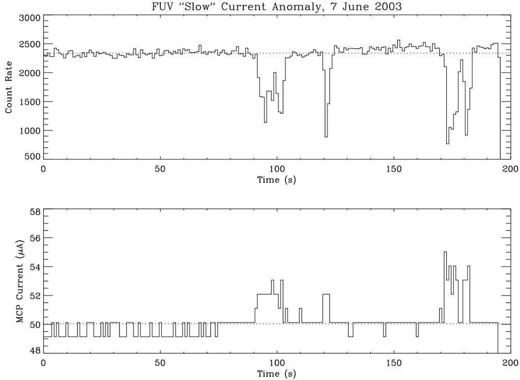
**Figure 6.** The anomalous FUV count rate and MCP current observed on 7 June 2003, about 5 weeks after launch. The global decreases in count rate are each correlated with few- $\mu\text{A}$  increases in HV current, and the slope of the count-rate-versus-current curve is the same for this data and the major 11 March 2005 anomaly, strongly suggesting the events are the same phenomenon.
