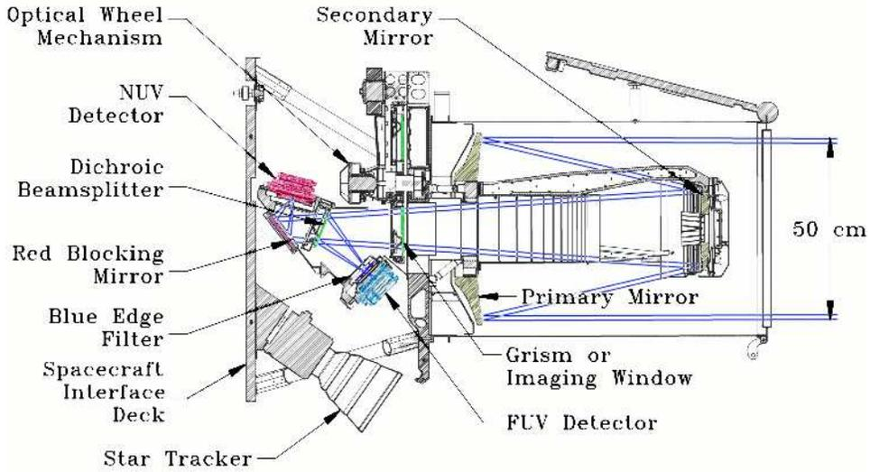
**Figure 2.** A cross section of the GALEX instrument showing 50 cm primary mirror, optics wheel, dichroic beamsplitter, red-blocking mirror, and a pair of photon counting microchannel plate detectors.
