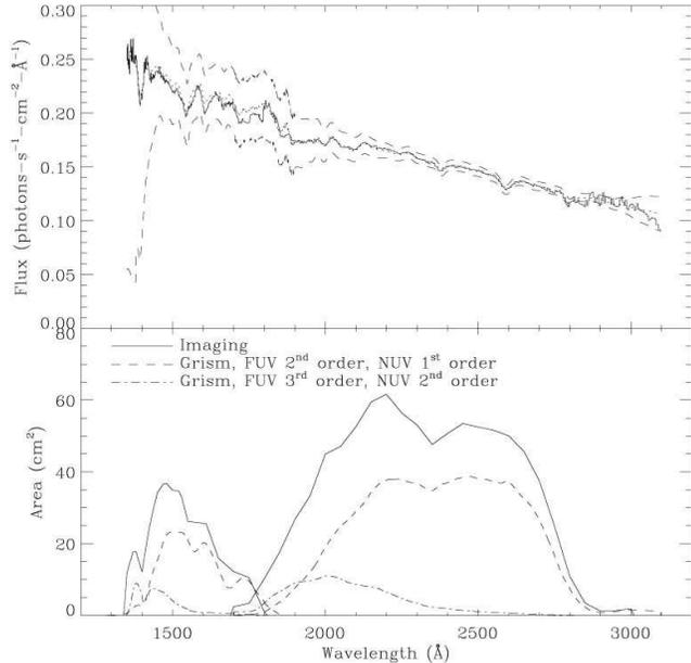
FIG. 3.— *Upper panel:* (Solid line) A composite of 42  $\sim 240$  s GALEX spectra of the *HST* white dwarf standard star BD+33°2642. (Dotted line) The *HST* reference spectrum. (Dashed lines) The range of  $1\sigma$  variations among the 42 spectra. *Lower panel:* (Solid lines) The ground-measured imaging-mode effective area. (Dashed lines) The flight-measured grism-mode effective area. (Dot-Dashed lines) The additional effective area in the grism 2nd (NUV) and 3rd (FUV) orders.
