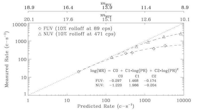
FIG. 2.— Local photometric non-linearity measured with white dwarf standards. Empirical fits are overplotted. The function parameters  $PR$  and  $MR$  correspond to the predicted and measured source rates, respectively.
